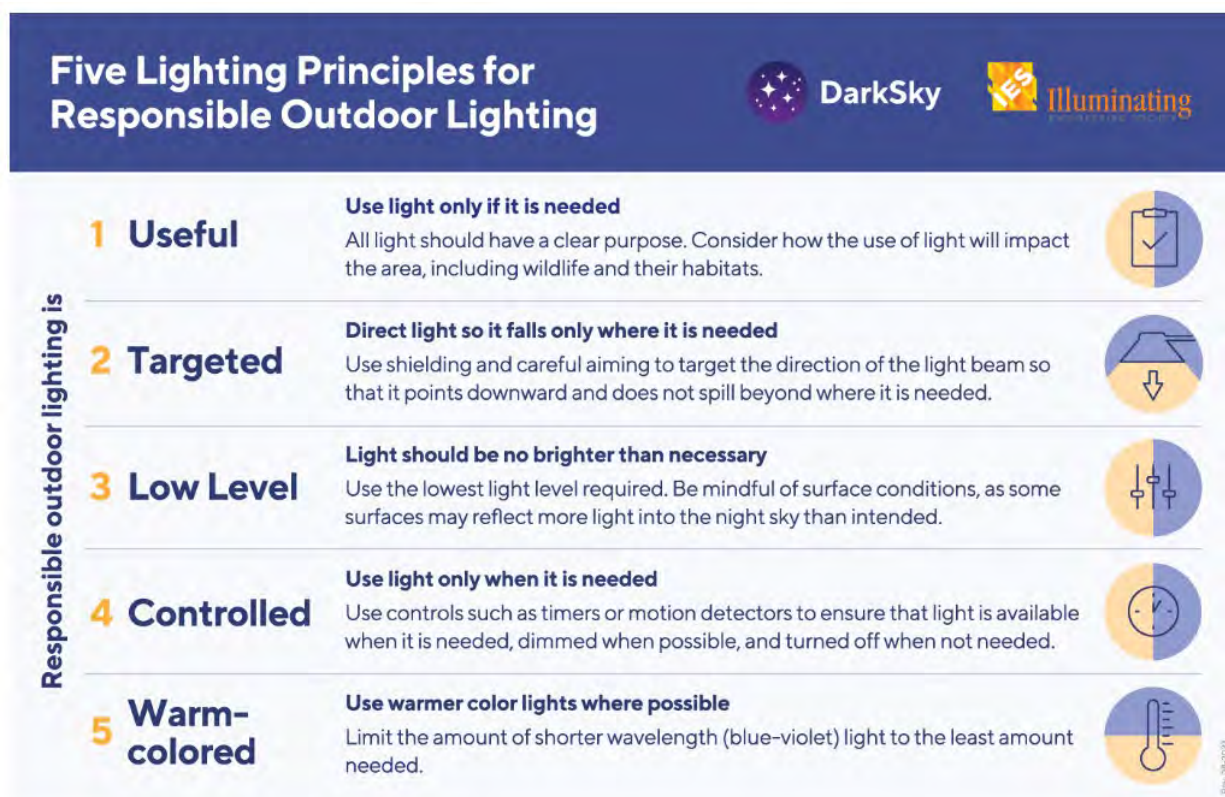
Figure 37. Dark Sky Lighting Principles for Responsible Outdoor Lighting
