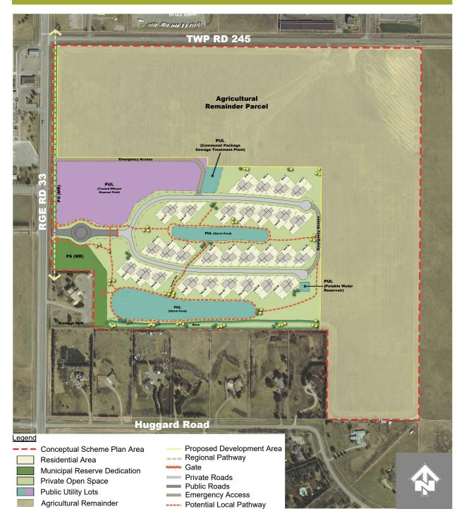
Given the relatively dense arrangement of housing within the Pradera Springs neighbourhood, the developer will accommodate a fire suppression system including installation of an on-site reservoir and pumping system to provide minimum fire flows to a pressurized hydrant system.
