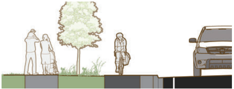
Figure 21: Separation from the sidewalk is valuable for reducing pedestrian use of the bicycle lane. The use of physical separation with vertical elements is one configuration. Image from the FHWA Small Town and Rural Multimodal Networks Design Guide.
