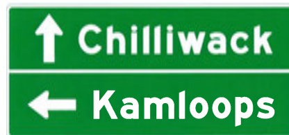
Figure 44. MUTCDC guide signs IA-2 or IA-3 can be appropriately scaled for active transportation users (refer to MUTCDC Table A1-5), and assembled with the IB-23 for bicycle navigation. Image from the MUTCDC A4.2.1.
