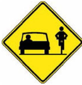
Figure 7: Share the Road Sign (WC-19 and WC-19S) can be used as cautionary signs. WC-19S is a supplementary tab sign used to convey the meaning of WC-19. Images from TAC Bikeway Traffic Control Guidelines for Canada 2nd Edition (4.6.7).
