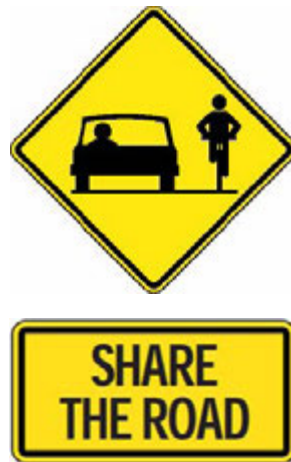
Figure 28: Share the Road Sign WC-19 and supplementary tab sign WC-19S can be used as cautionary signs with advisory lanes. Images from TAC Bikeway Traffic Control Guidelines for Canada 2nd Edition (4.6.7).
