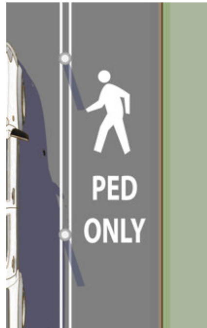
Figure 33: Pavement markings for pedestrian lanes. Image from the FHWA Small Town and Rural Multimodal Networks Design Guide pg 5-7.
