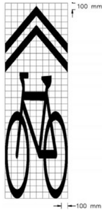
Figure 42: Shared use lane symbol from TAC Bikeway Traffic Control Guidelines for Canada.
