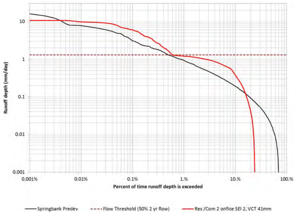
Figure 4. Residential / Commercial (Pond with 2 Orifice) flow duration curves
