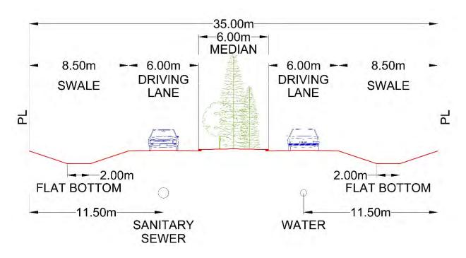
Figure 6: Proposed Modified Road Cross-Section for Strawberry Hills Gate
