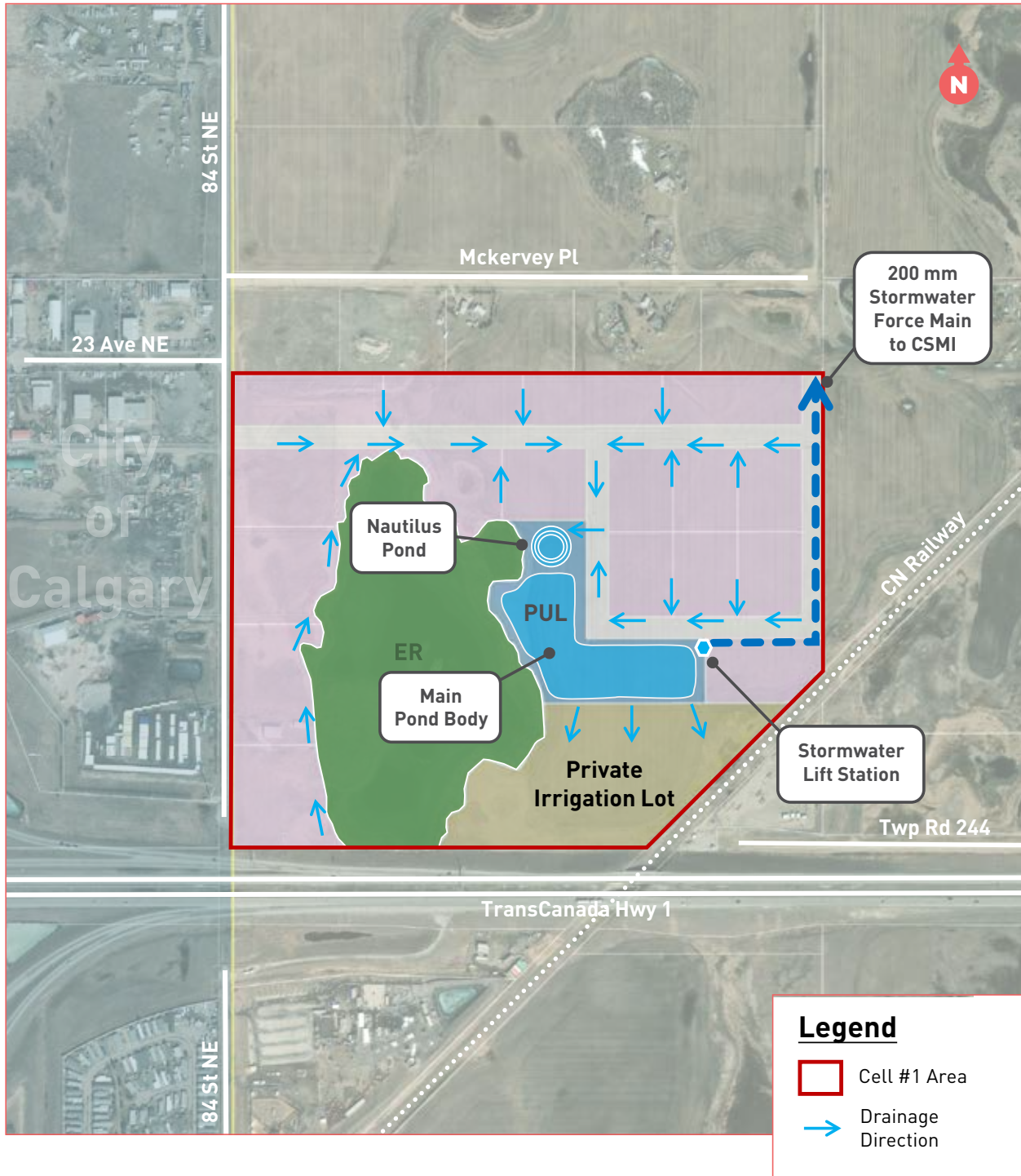
Figure N°12a CELL #1 STORMWATER MANAGEMENT
