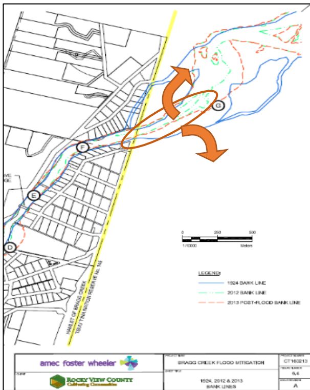
Figure 1: After Application Appendix C, Figure 6.4. Shapes in orange added to identify potential overtopping area (orange oval) and direction of flooding (orange arrows).
