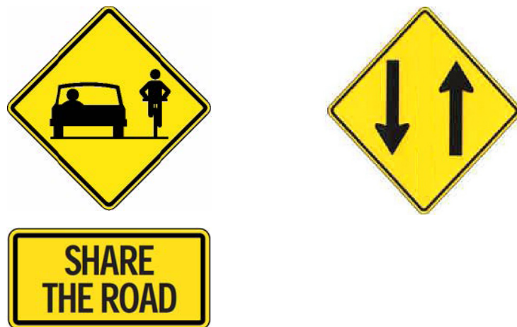
Figure 37: Share the Road Sign WC-19 and supplementary tab sign WC-19S can be used as cautionary signs. Images from TAC Bikeway Traffic Control Guidelines for Canada 2nd Edition (4.6.7).
