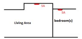
4) <u>Bulkheads</u> – Where a bulkhead is framed into a ceiling, such as in a basement area, a smoke alarm can be located on the underside of the bulkhead, on the ceiling, or on the top 300mm (12") of the wall.
