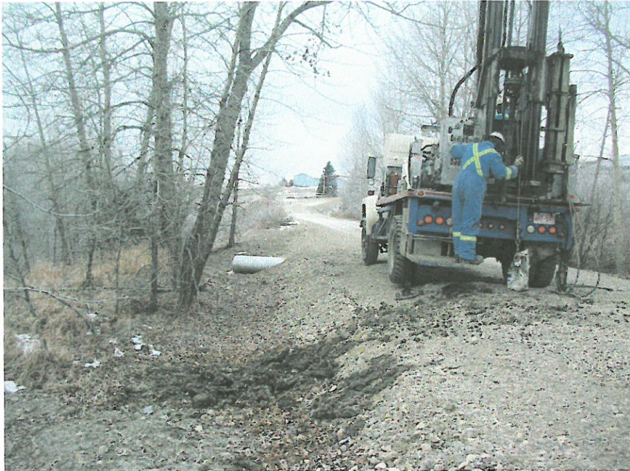
Photo 7: View of drill set up on TH3, centre slide. Note approximately 1 m high roadway fill over down dropped slide block, (Dec 05) .
