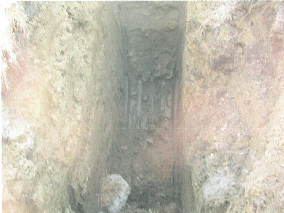
Photo 4: Test pit through silty clay on lower part of east slide, (Dec 05).
