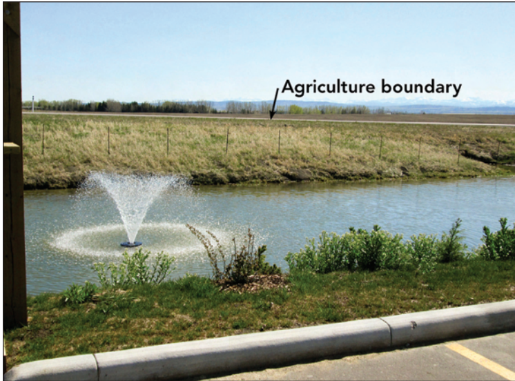
Place stormwater ponds between principal buildings and the boundary to create a buffer and serve as an amenity.
