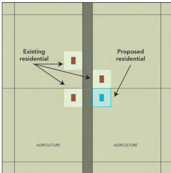
In this example, the design tools have been implemented by locating the new home near existing homes, in a corner, and creating only two new boundaries with agricultural land.
